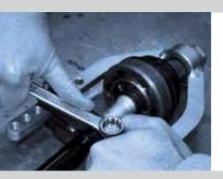
After removing the driveshaft from the steering knuckle, attach the joint puller to the driveshaft. Make sure a sufficiently large free area is left on the bolt threads so that the joint can be loosened from the safeguard and the nut does not stick to the keyway.
