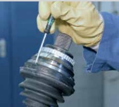
Fill 2/3 of the grease provided in the repair kit into the boot and the remaining grease into the joint.
