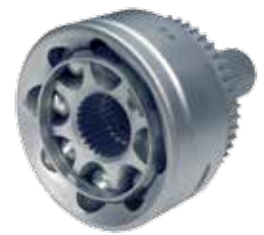
Fixed ball joint (SX) featuring Countertrack™ technology
